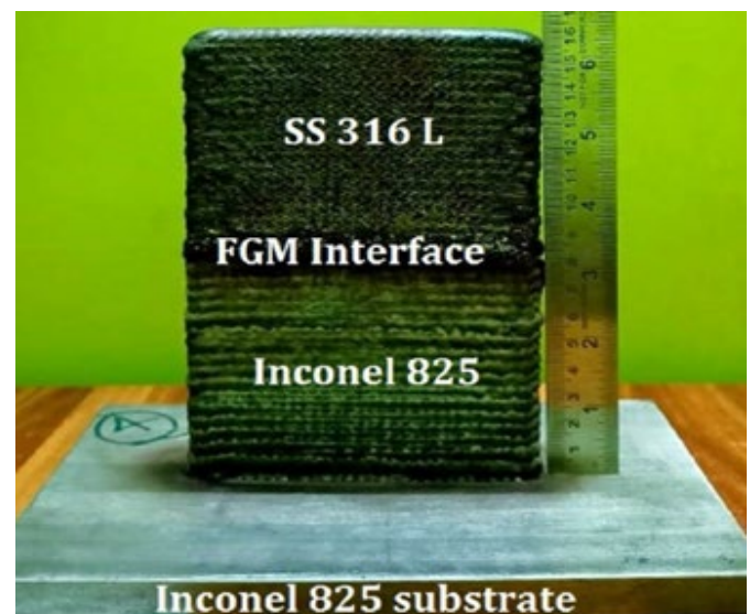
Figure 3 Building of the FGM with WAAM [22]
