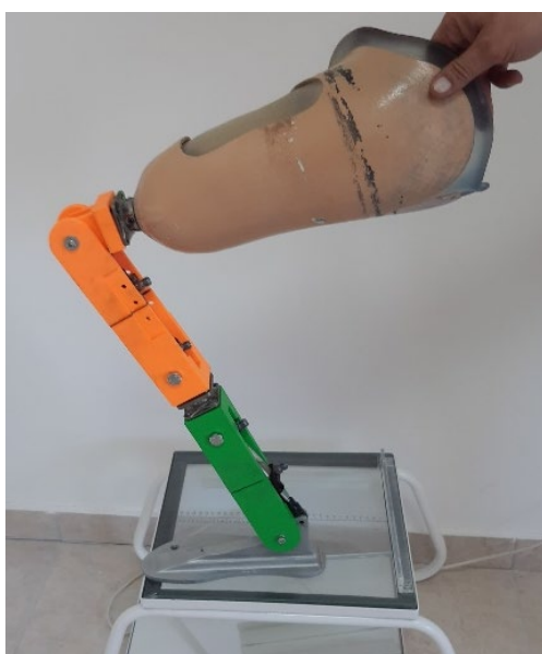
Figure 9 The first attempt at applying additive technology in the creation of a transfemoral prosthesis
