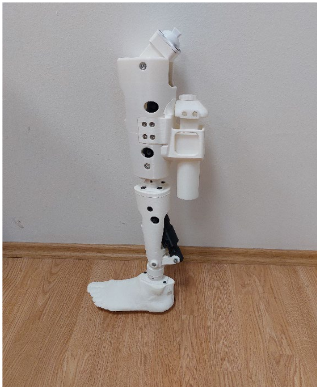
Figure 16 The final assembly of the above-knee prosthesis
