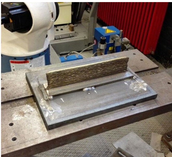
Figure 1 Final appearance of the deposited WAAM wall
